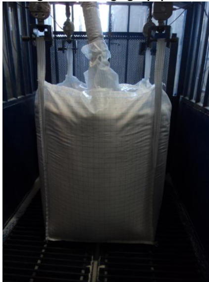
Sun-Stat FIBC on Properly Grounded Filling and Discharging Equipment
